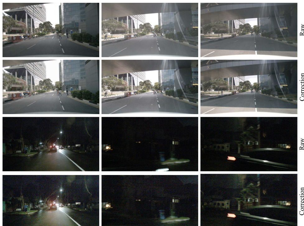
Fig. 6 Qualitative comparison of images before and after Spatial-temporal Photometric Consistency Correction. The top two rows illustrate the correction effect on three temporally adjacent images. The bottom two rows demonstrate the correction effect on spatially adjacent images captured in nighttime conditions. For optimal details, viewing with zoom-in is recommended
